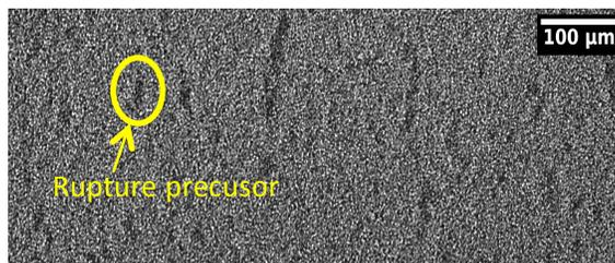
Microscopy image of a colloidal gel damaged by accumulation of strain oscillations
